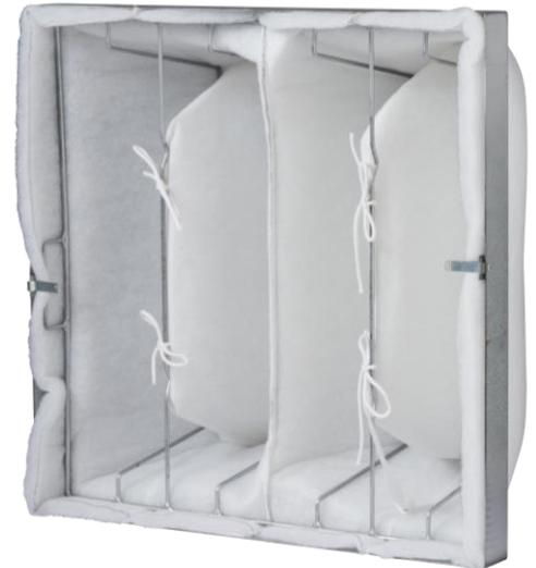
1. The Main Mounting or Fixed Frame, incorporates a specially designed wire "Media Support Frame". This frame ensures that the media does not vibrate or flap when in use, or sag when the system is turned off, thus preventing accumulated dust from vibrating loose and passing into the air stream on start-up.
